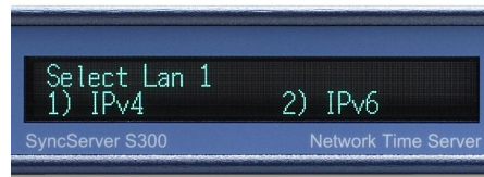
Crisp and bright vacuum fluorescent display offers high readability both near and far. Characters can be large, medium or small. Intensity is user adjustable.
